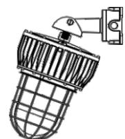
4. Connect the AC cable. Black cable connects to L. White cable connects to N. Green cable connects to grounding.
